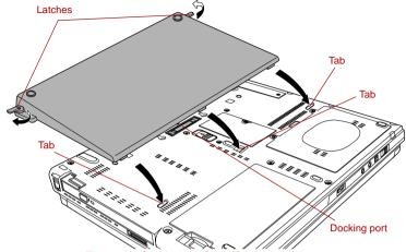
Figure 6-4 Seating the Slice Expansion Battery
